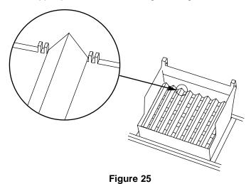
The open "U" of the cooking grates goes down. Set the cooking grates onto the ledges in the cooking box. Figure 26.
